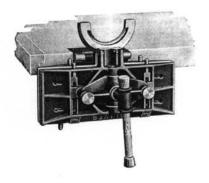
Fig. No. 8 Showing use of steel faced jaws
