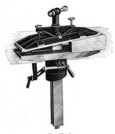
Fig. No. 5 Jaws horizontal, clamping angle piece
