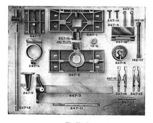
Fig. No. 2 A demonstration of the fact that "Oliver" No. 1 Universal Vise has fewer parts than any other similar vise.
